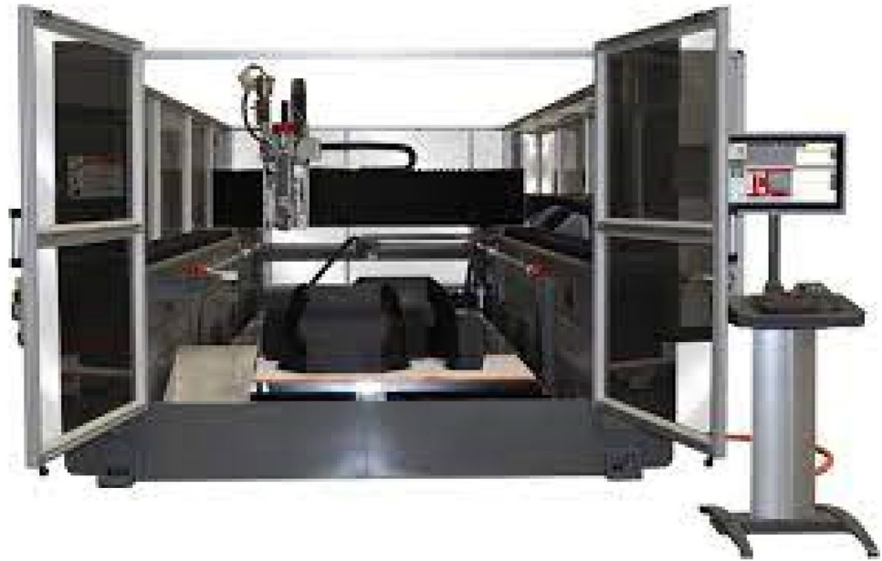
Fig. 2 BAAM system (Cincinnati Incorporated)
