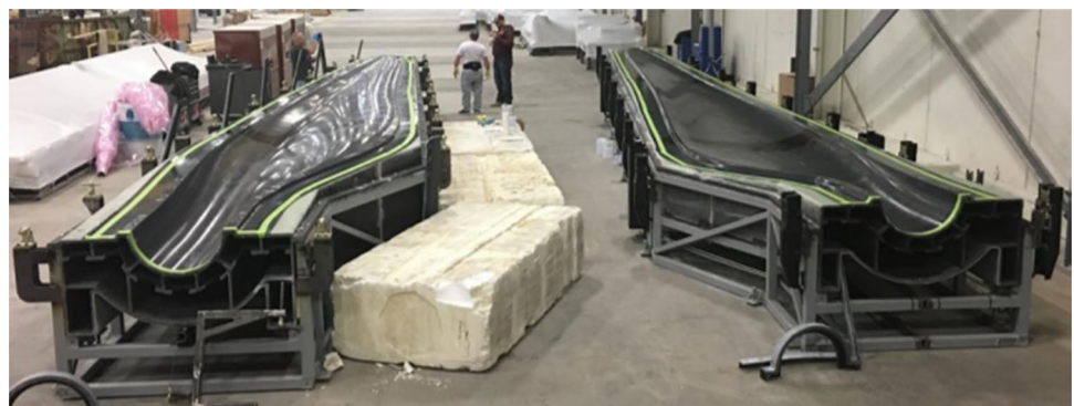
Fig. 10 3D printed wind turbine mold by ORNL [88]
