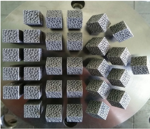
Fig. 6 Photo of the cp-Ti lattice samples grown on the platform in the plane, edge and corner orientations (from left to right)
