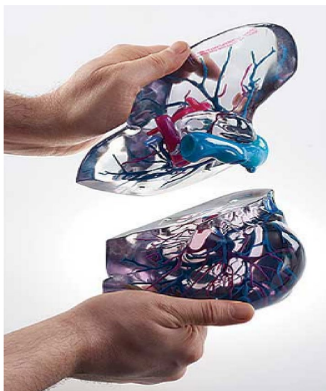
Fig. 3 Liver produced by additive manufacturing [17]
