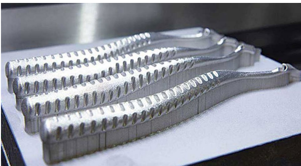
Fig. 22 These surgery guides for ACL repair were printed with Inconel 718 by DMLM [17]
