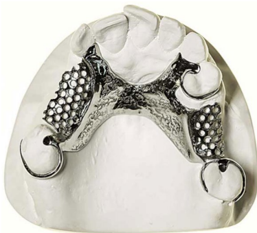
Fig. 11 Dental device manufactured by additive manufacturing [17]
