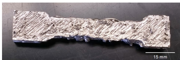
Fig. 18 FFF 3D-printed ASTM E8 standard tensile specimen of Sn60Bi40 alloy
