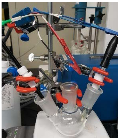
Fig. 2 Electrochemical corrosion studies setup used in this study
