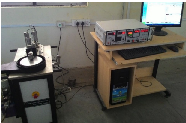
Fig. 3 Pin-on-disc wear test experimental setup
