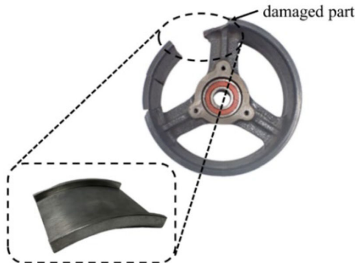
Figure 1. Damaged pulley and cut-out specimen (a) EN-GJL-250 (b) Abnormal EN-GJL-250.
