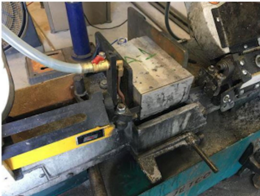
Figure 4. Cutting of cast composite material.
