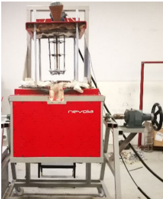
Figure 1. The furnace used in casting process.
