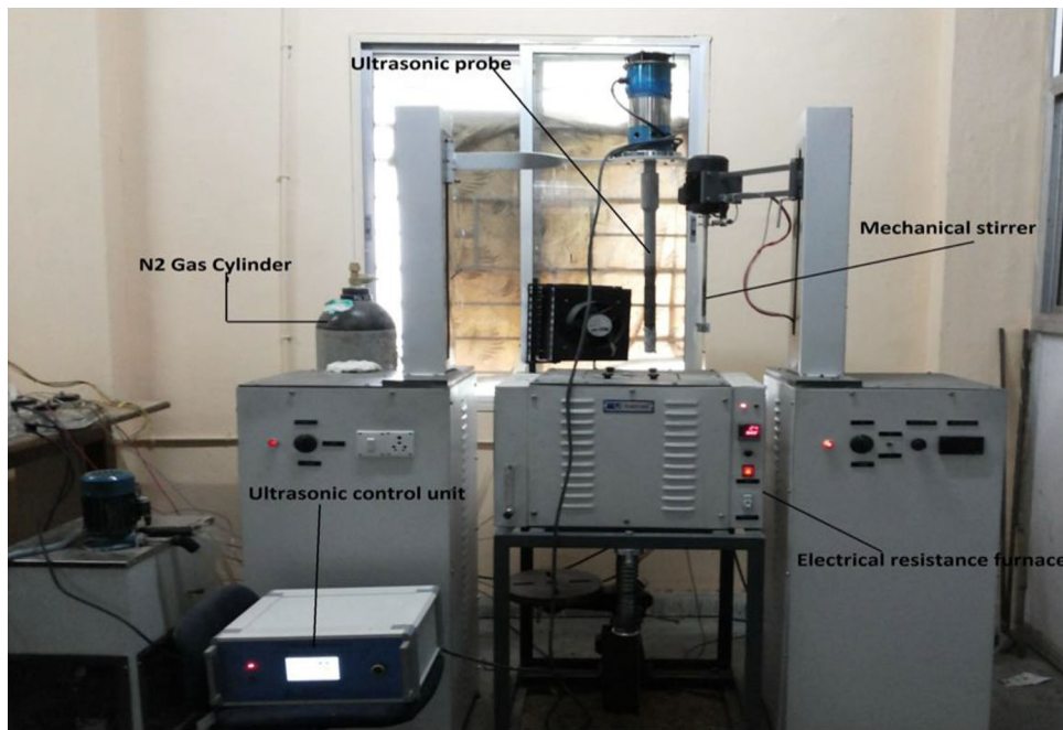
Figure 1. Stir-squeeze casting setup assisted with an ultrasonic probe.
