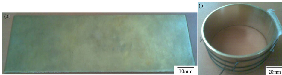
Fig. 1. The preparation process of a brass hollow cylinder; (a) Brass sheet cut out to 265 \times 40 \times 3 \text{ mm}^3 dimensions and (b) Brass sheet formed into a cylindrical shape and closed using asbestos and steel wires.
