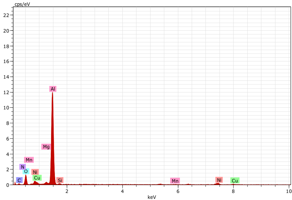
(e3): EDAX spectra showing elements present in ON40 alloy composite
