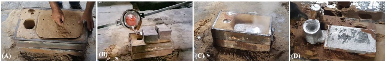
Figure 5. DWS processing steps, (a) cap assembly and venting, (b) pouring, (c) cap withdrawal and spraying, and (d) mold collapsing and removing the casting.
