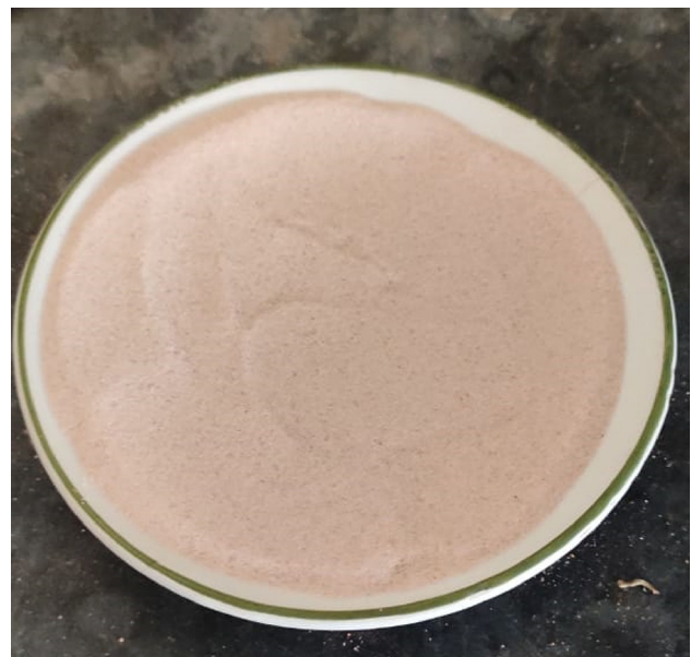
Figure 3. Printed sand heated at 600 °C.
