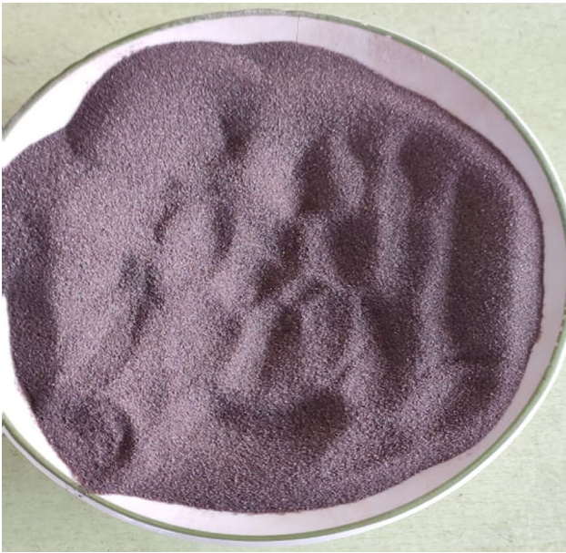
Figure 4. Printed sand heated at 400 °C.
