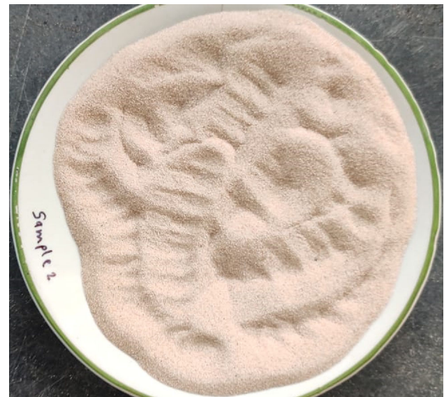
Figure 11. Unprinted sand heated at 500 °C.
