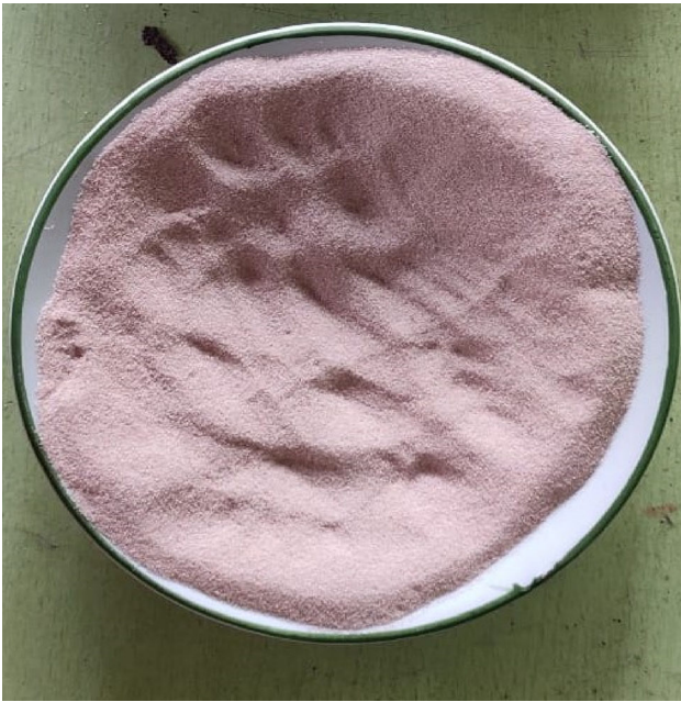
Figure 8. Unprinted sand heated at 800 °C.
