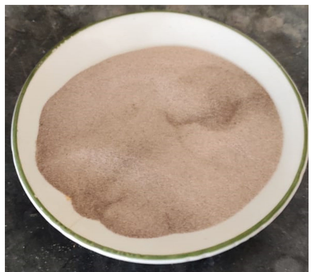
Figure 7. Printed sand heated at 450 °C.
