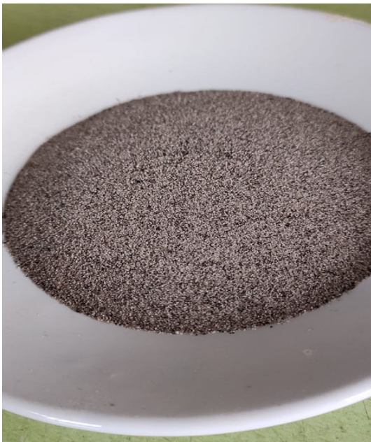
Figure 9. Unprinted sand heated at 200 °C.
