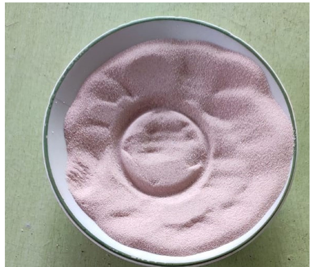
Figure 2. Printed sand heated at 800 °C.
