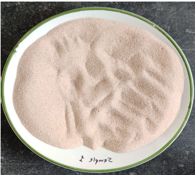
Figure 5. Printed sand heated at 500 °C.
