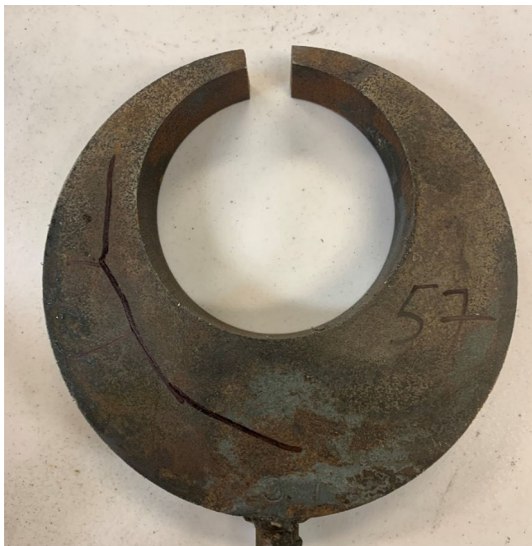
Figure 6. Crack in ring 57, another crack is present with 180° symmetry to this crack.
