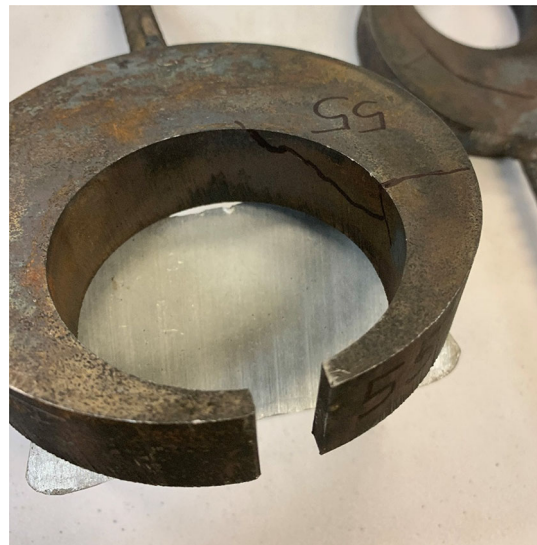
Figure 7. Crack in ring 55. Unlike ring 57, there is not a symmetrical crack present.
