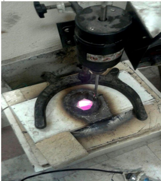
Figure 2. (a) Ultrasonic probe and (b) mechanical stirrer and ultrasonic device.
