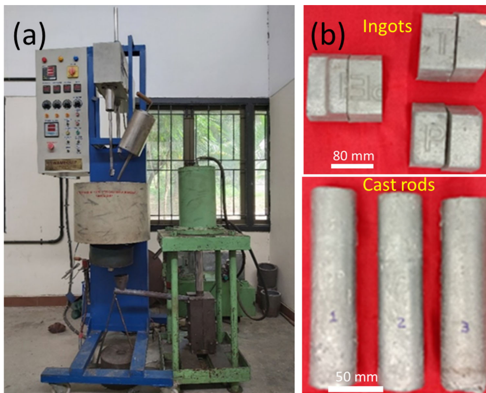
Figure 3. Photograph of: (a) Stir cum squeeze casting setup; (b) A356 ingot and cast samples.
