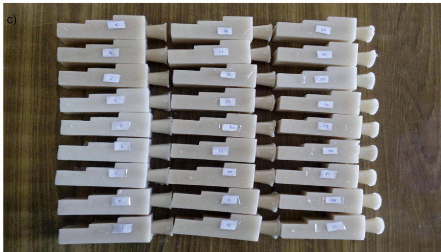
Figure 1. (a) Wax injection machine, (b) geometry of wax pattern, (c) wax blend patterns.
