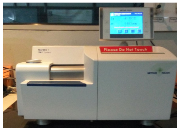
Figure 3. Differential scanning calorimetry (DSC) setup.
