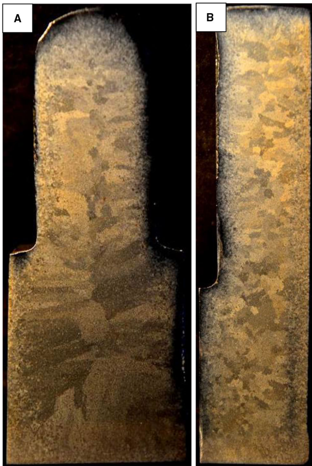
Figure 8. Solidification macrostructures of Melt B, shape SA (a) and SC (b).
