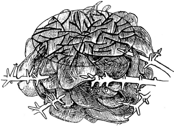
Figure 1. Drawing of eutectic cell graphite with interpenetrating austenite dendrites by Morrogh and Oldfield. 1
