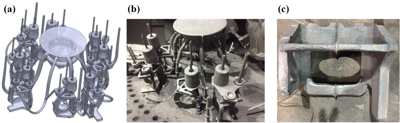
Figure 7. (a) 3 DSP featured freeform-based rigged model of nested complex bracket casting: Iteration 2. (b) Experimental cast part from second iteration after the mold is shaken out. (c) One of the eight cast parts after the parent casting from second iteration is cleaned off risers and in-gates.
