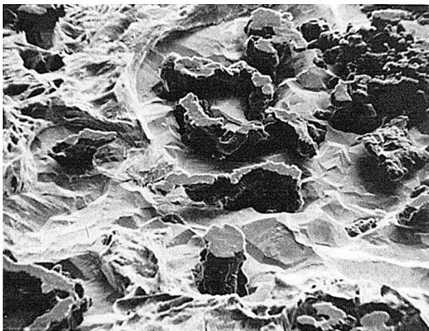
Figure 36. Deep-etched transition zone in fast-cooled high-purity Fe-C-Si alloy. 53
