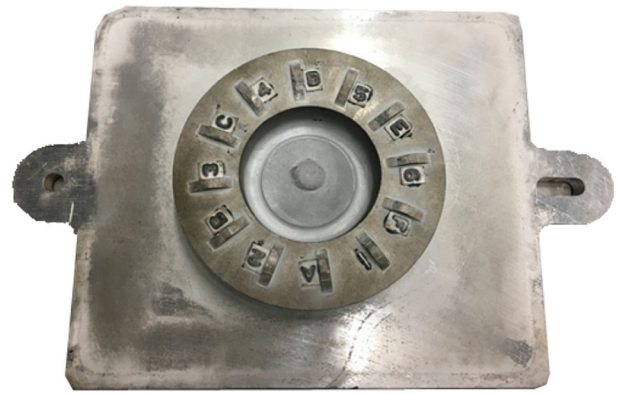
Figure 4. Matchplate pattern for the surface defect casting trial.
