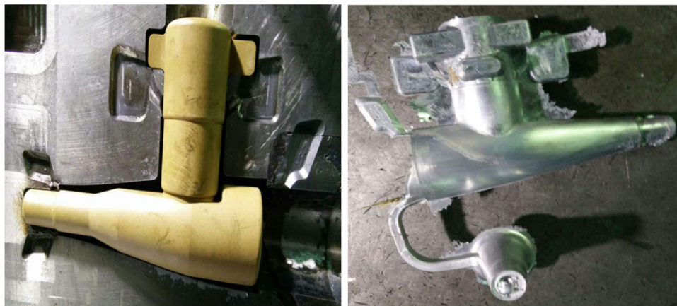
Figure 1. Photographs of “triplet” salt core and “triplet” die casting blank.
