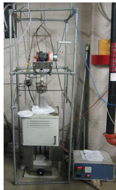
Figure 14. Experimental LIBS probe (with furnace) developed by the Energy Research Company. 73
