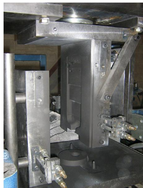
Figure 1. The mold is mounted on LPPM press.
