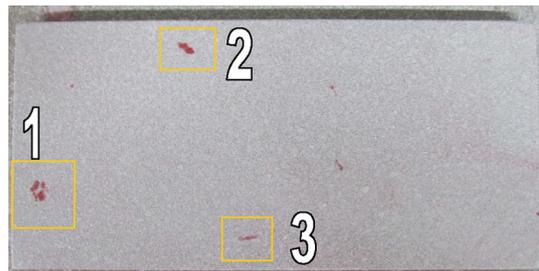
**Figure 9.** A dye check on the machined surface of the 25 mm plate, 80 × 160 mm (3.15 × 6.30 in.) (casting #5) is shown.
