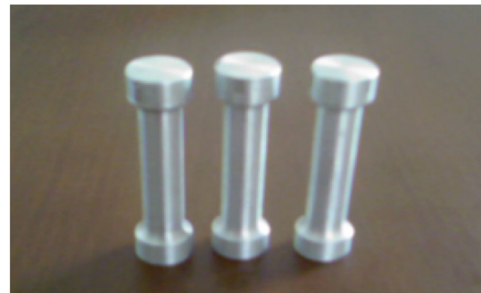
Figure 23. Three high-pressure die-cast tensile test specimens ready for testing.
