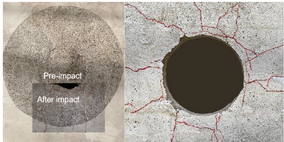
Fig. 11 Model failure after impact
