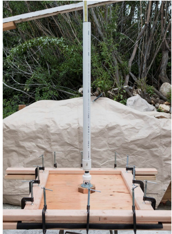
Fig. 4 The horizontal fracture grouting assembly
