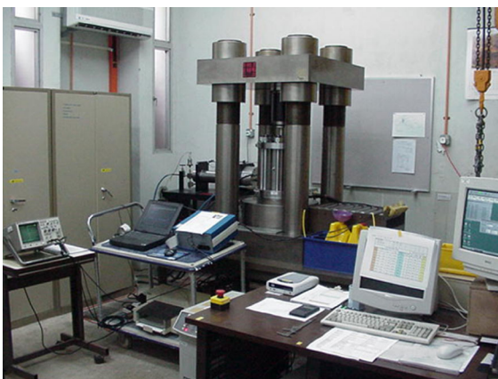
Fig. 3 Overview of triaxial compression testing system
