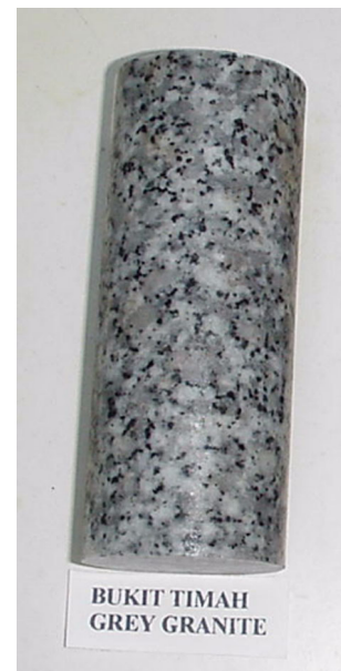
Fig. 2 Prepared rock specimen for testing
