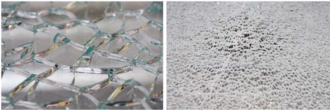
Fig. 1 Fragmentation of tempered glass. Left: low residual stress state. Right: high residual stress state
