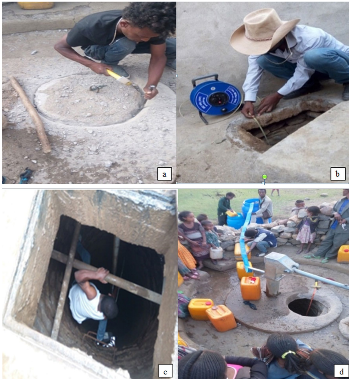
Fig. 4 Measurement procedure for water yield and static water level of hand-dug wells: a digging manhole, b measuring water level, c measuring diameter of the well, and d pumping water
