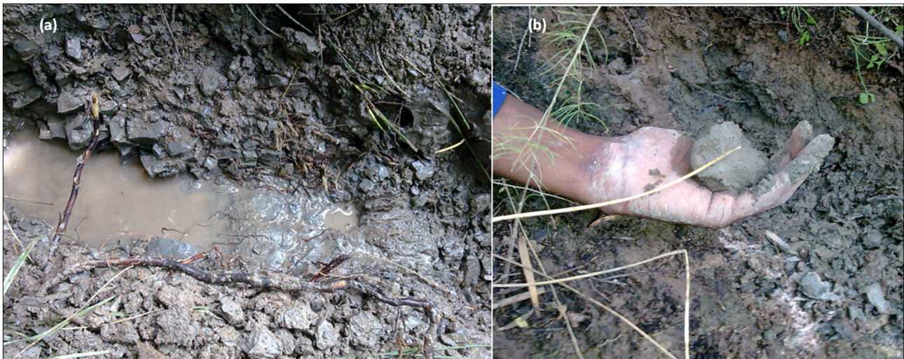
Fig. 10 River cut-bank photographs of a saprolite and b silty clay overlying the saprolite
