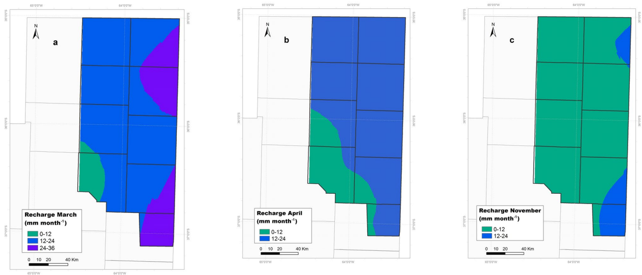
Fig. 7 Maps of recharge ( \text{mm month}^{-1} ) for: a March, b April, and c November
