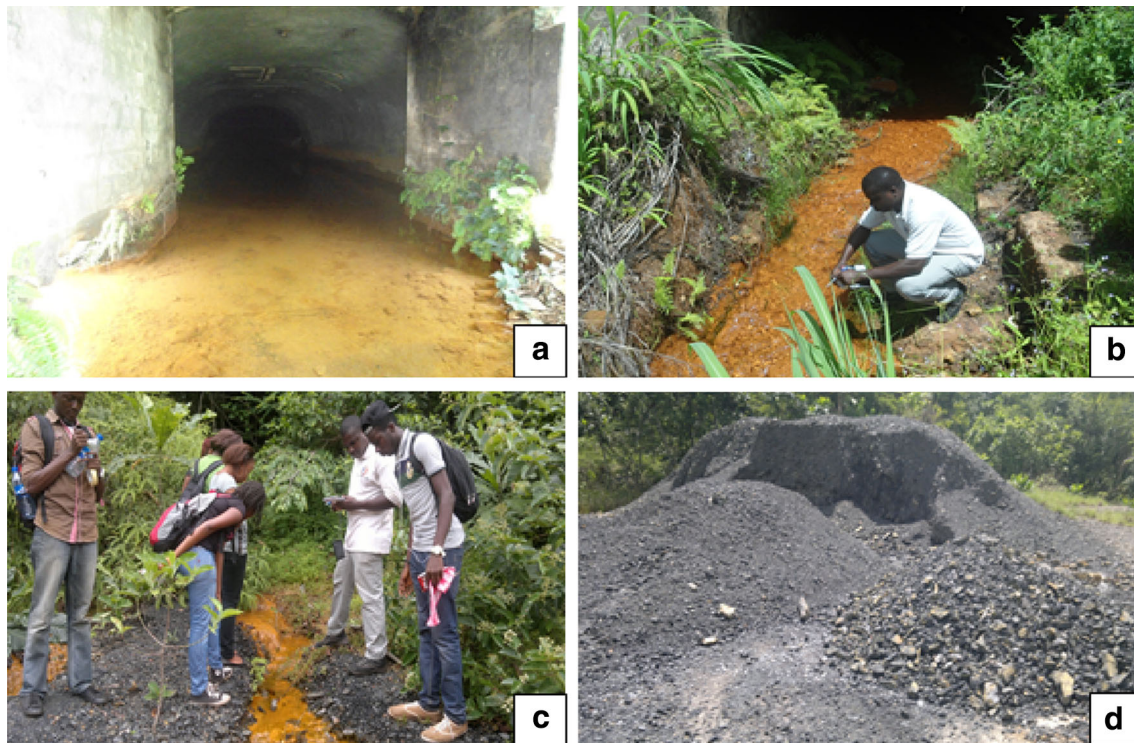
Fig. 7 Water flowing out of a mine tunnel which intercepts the water table at the Iva Valley coal mine (a, b) through and over surface mine waste dump site (c) scattered indiscriminately over the study area (d)
