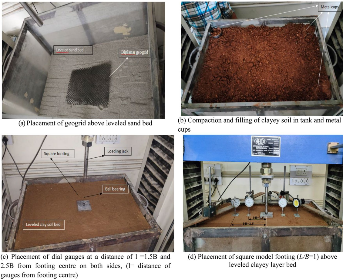
Fig. 5 Preparation of model plate load test set up
