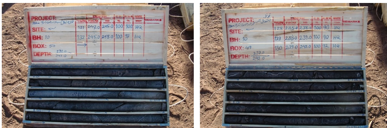
Fig. 5 Core samples of the drilled boreholes in the zone HG11
