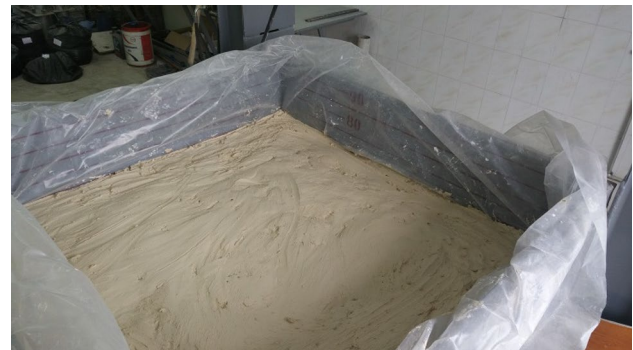
Fig. 6 Preparation of the kaolin clay bed in large test box
