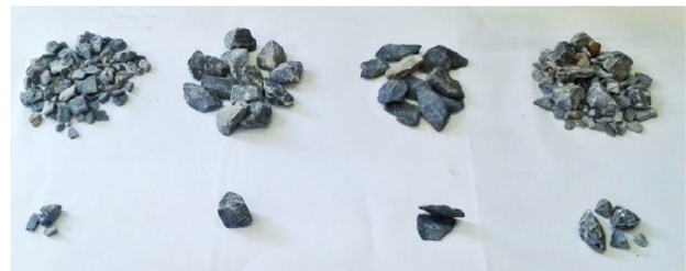
Fig. 17 Different gravels ( G1 fine-grained gravel, G2 sub-angular gravel, G3 flaky gravel, G4 mixture of G1 and G2 )
