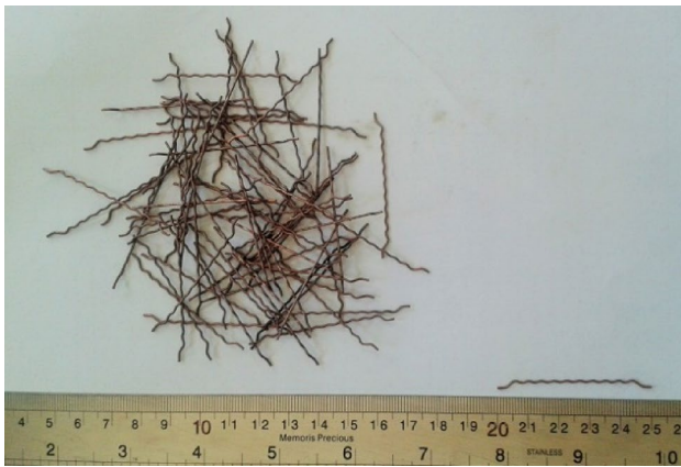
Fig. 7 Steel fibre reinforcement
