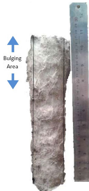
Fig. 20 Deformation of single stone columns
