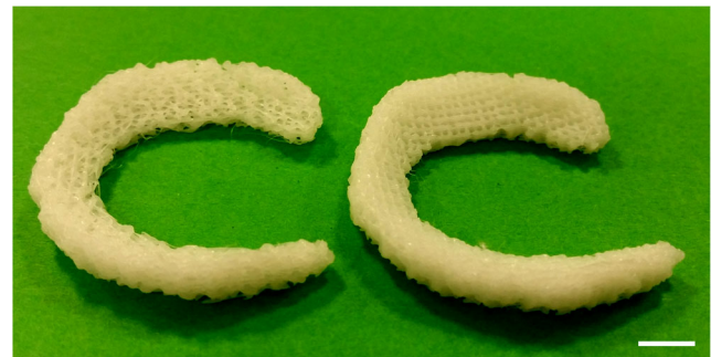
Fig. 9 3D-printed patient-specific scaffolds from polycaprolactone with different internal architectures using the 3D meniscus model that was obtained from the patient's high-quality MRI volumetric image dataset. The scale bar indicates 1 cm.
