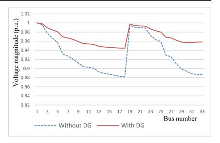
using LSE in DG interconnected distribution network and it is tested and verified. Voltage profile improvement is observed by placing the DG in the system. A comprehensive LSE algorithm is evolved, tested, verified and reported considering different aspects of a modern day electric distribution network.
