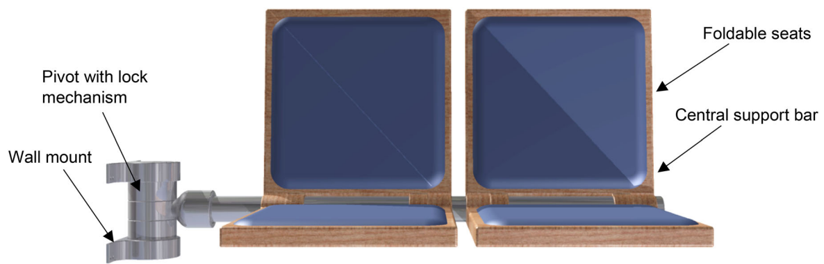
Fig. 15 Transverse folding seat design
