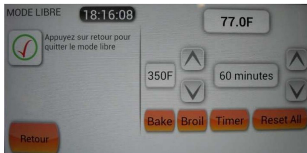
Fig. 5 The free mode enabling to manually control the smart cooker
