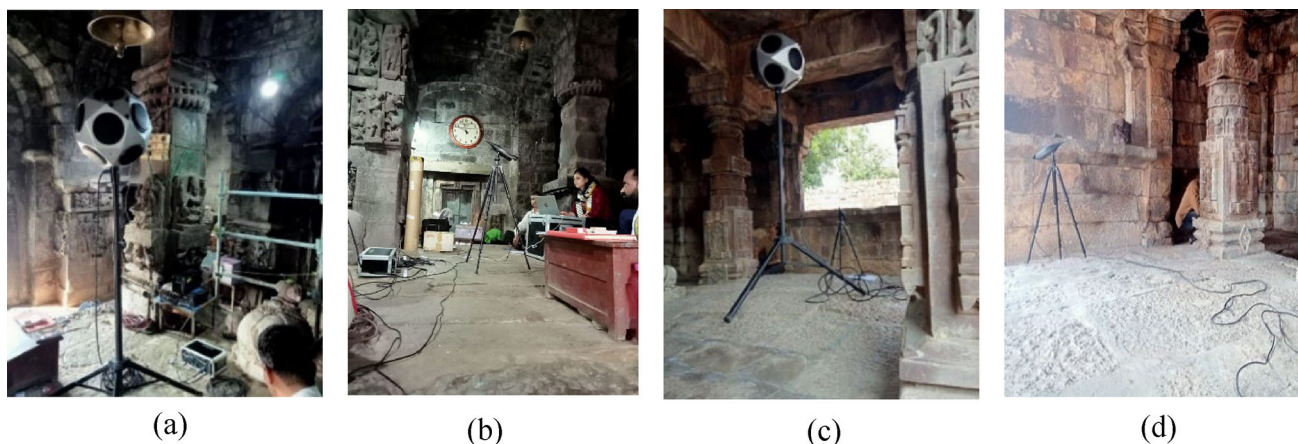
Fig. 6 a Markanda temple sound source (S1) (center of the pavilion) b Markanda temple receiver position (S1) (center of the pavilion) c Mrikunda temple sound source (S1) (center of the pavilion) d Mrikunda temple receiver position
