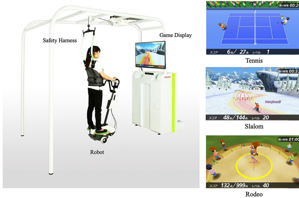
Fig. 1 The system of the balance exercise assist robot (BEAR). The BEAR system consisted of a robot (boarding equipment), a game display, and a safety harness. A rider moved the robot and controlled his/her avatar in the games. The robot consisted of 2 steps with the load sensor, 2 wheels with in-wheel-type motors, and a handle attached to the center pillar. The robot maintained a horizontal position by itself
