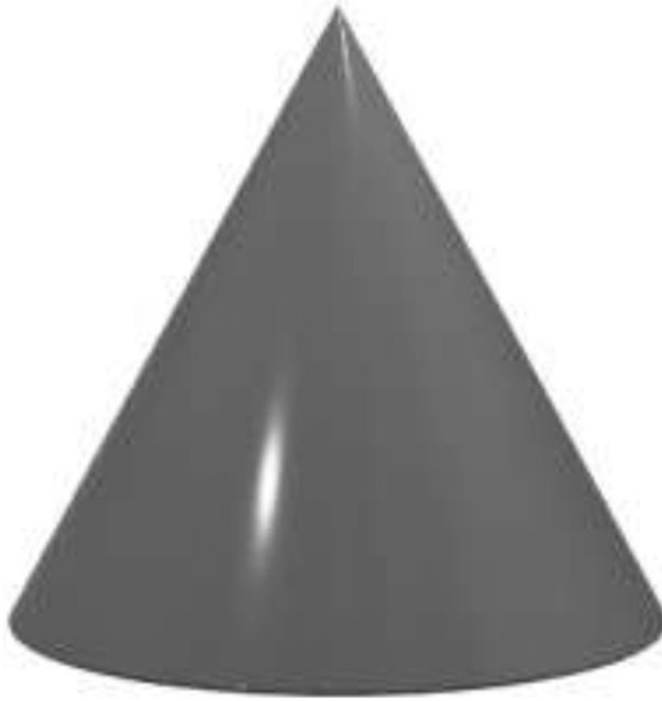
Fig. 9 A schematic illustration of a summit. At the summit, the surface openness is positive, because all the surroundings are lower than the summit
