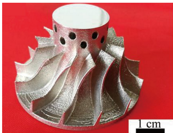
Figure 13 Small turbine blade manufactured via SLM. Reprinted with permission from Ref. [34], Copyright 2019, Elsevier.
