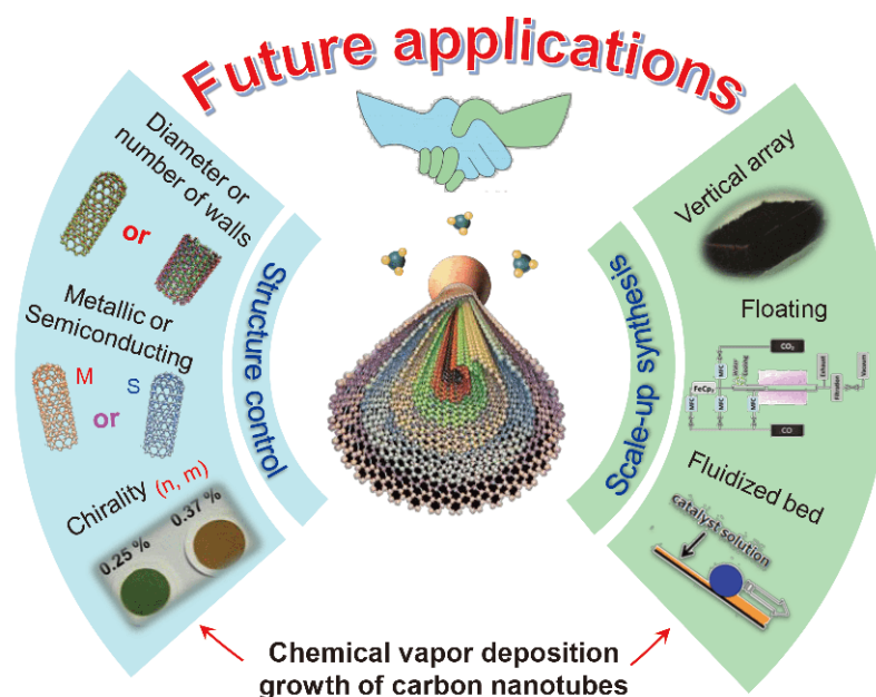
Figure 8 Future design for CVD growth of CNTs in industrialization. Fine structure control should be combined with scale-up synthesis, and this will determine the killer applications of CNTs.
