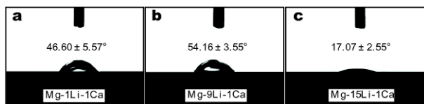
Figure 10 The CAs of the (a) Mg-1Li-1Ca, (b) Mg-9Li-1Ca and (c) Mg-15Li-1Ca.
