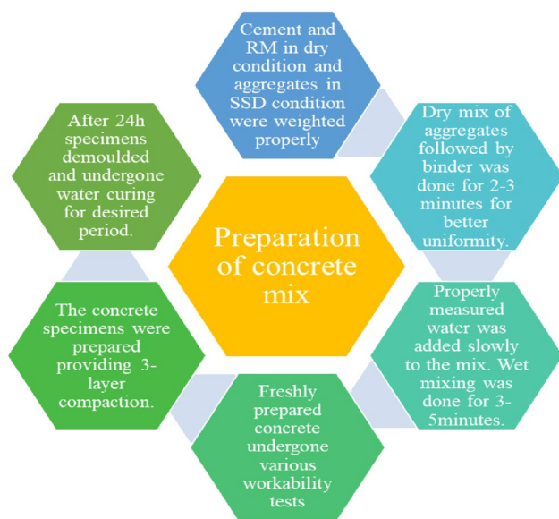
Fig. 1 General preparation procedure of concrete mixes
